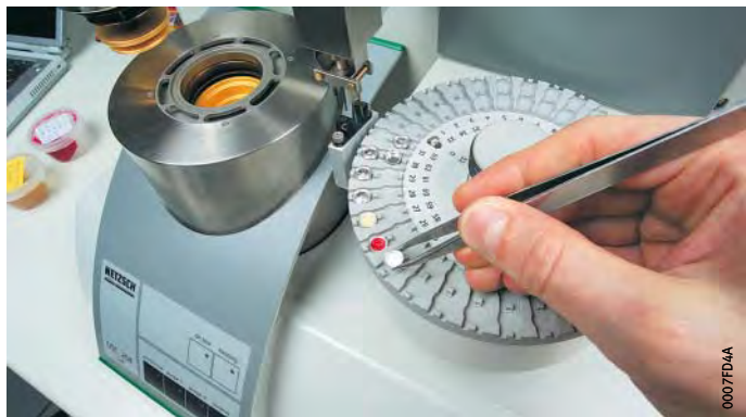
Figure 6 Analysis of the thermal behaviour of greases
