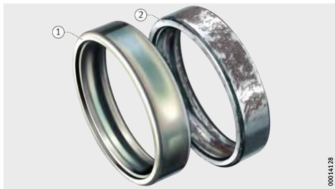
Figure 8 Bearing rings after the salt spray test
