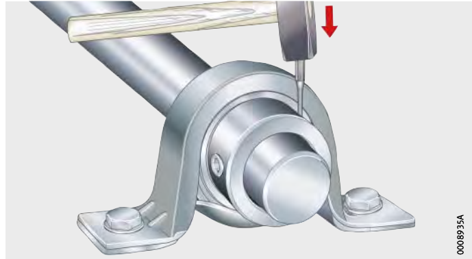
Figure 13 Tensioning the eccentric locking collar
