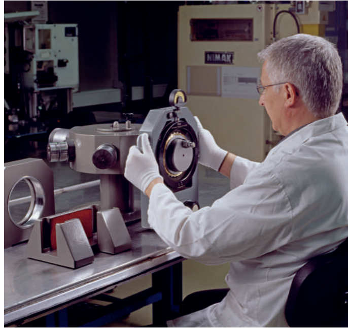
34 Positioning the enveloping circle gauge
